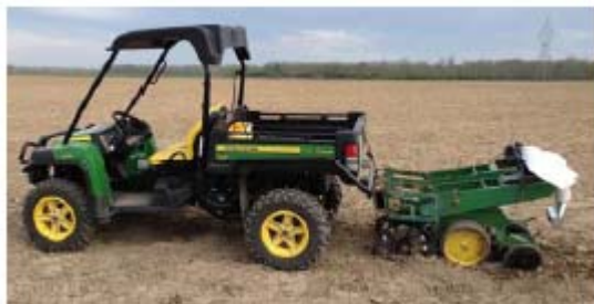
Figure 12. John Deere Gator™, two-row mock-planting unit and dust collection device.
