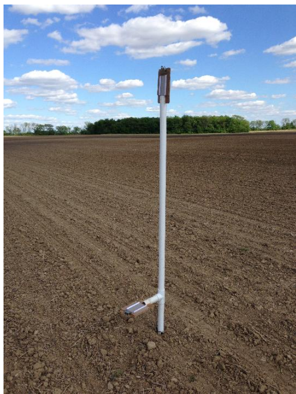
Figure 1. Dosimeter used for collecting seed treatment dust drift during planting trials. Five microscope slides coated with Tanglefoot adhesive are placed in a horizontal orientation 30cm above the surface of the field and in a vertical orientation 2m above the surface of the field.
